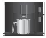
When the IMPRESSA is switched off, the system is automatically rinsed if a specialty coffee has been prepared.
