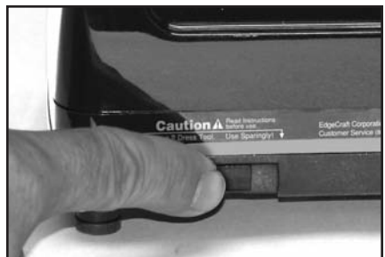
Figure 11. Cleaning the polishing disks (see text).
