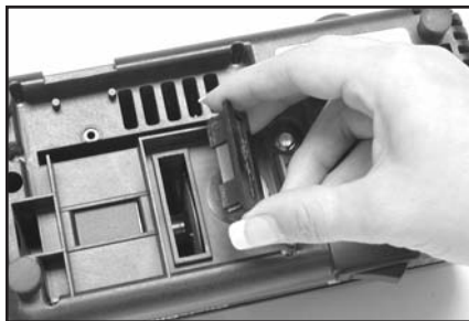
Figure 12. Removing cover under base to clean out metal dust. (See Normal Maintenance section)
